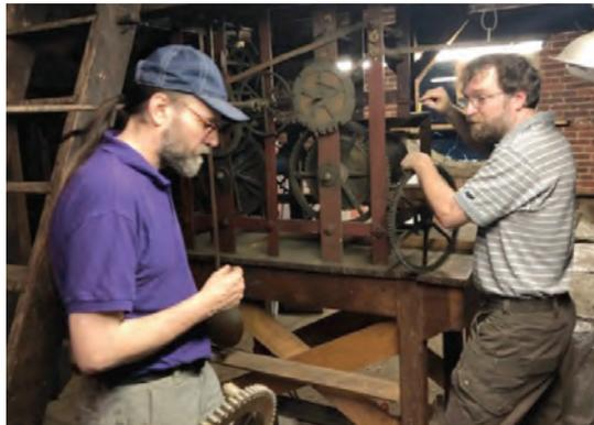
**Headhouse clock being disassembled and inspected**
