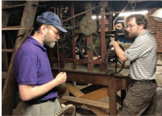
**Headhouse clock being disassembled and inspected**
